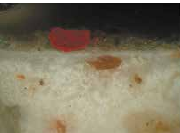
Sample T-2: microphotography in reflected white light (clear section, 500X)
