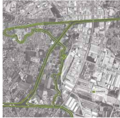
levees store and direct flood water to protect property within the Roncajette park area
